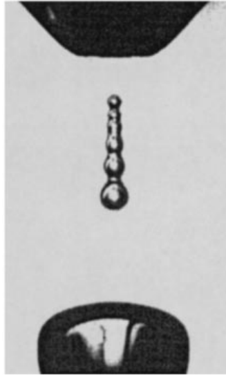
FIGURE 13. High-speed ciné camera image of a pendant drop and its satellite: orifice plate radius, 3.85 mm; orifice material, precision ground glass; liquid, pure distilled water; drop volume falling away, 0.0991 ml; time after breakage of lower end, 2.8 ms; camera speed, 2500 frames s^{-1} .
